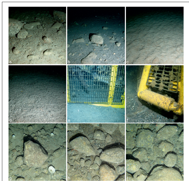
FIGURE 2 | Seabed environment and anthropogenic impacts surrounding Protective Structure A at Lancaster-205/21a-6; (a) undisturbed seabed with boulders, (b) boulders impacted by drill cuttings, (c) undisturbed coarse sand, (d) sand covered by drill cuttings, (e) base of the protective structure in contact with the seabed showing no scouring, (f) scoured sediment on the north west corner of the protective structure, (g–i) examples of background hard substratum from the 2011 environmental baseline survey, note Porifera in all images.
